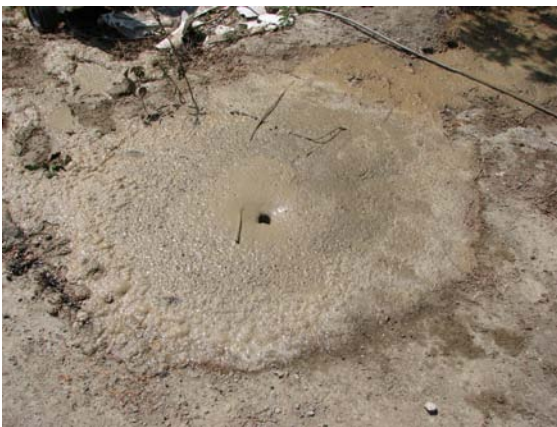
Chemical oxidation reaction of OxyTek-L™ in soil
